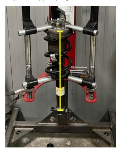
14. Compress the spring until tension is relieved from the strut. Remove the 18mm top nut and top mount. You will use the mount with your new Belltech coilover.
