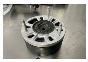
24. Assemble the spring bearing, helper spring, intermediate ring, main spring, upper spring seat, and the OE top mount onto the Belltech coilover.
