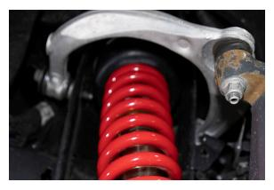
27. Attach the lower strut mount to the lower control arm using the supplied bolts, washers and Nyloc nuts. Torque the supplied nuts to 60 ft lbs.
