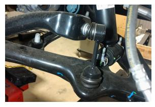
12. Push or pry down on the lower control arm to gain clearance and remove the strut from the vehicle.
