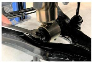
28. Attach the end link to the lower control arm, torque to 74 ft lbs. when the suspension is loaded or the vehicle is back on the ground.
