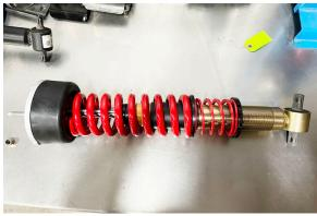
25. Reference the OE strut markings and ensure the top mount is oriented in the same direction it was before disassembly. Torque the supplied Nyloc nut onto the strut to 37 ft lbs.
