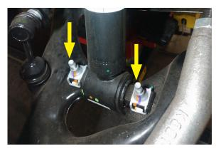
11. Remove the 18mm nut holding the anti-sway bar end link to the lower control arm. The nut is located on the underside of the lower control arm. This will allow the lower control arm to swing down and ease the removal of the strut.
